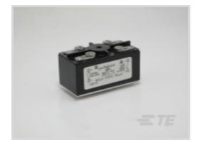
Power Relay Type: Solid State Coil Voltage Rating: 3.8 VDC Contact Arrangement: 1 Form A (NO) Contact Current Rating (Max): 10 A Contact Switching Voltage (Max): 250 VAC
